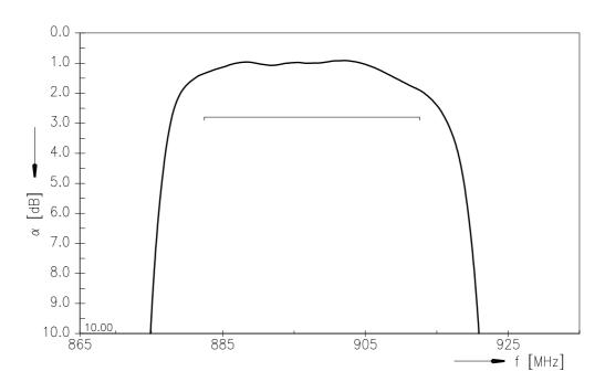
Frequency Response TX-ANT (Passband, CW test signal)
